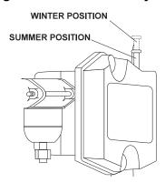
When the heat riser is in the SUMMER (down) position (Figure 2.2), air is drawn into the air cleaner from the upper intake tube.
